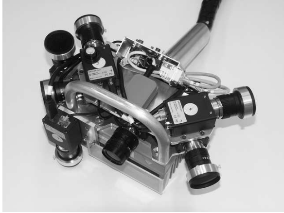
Figure 3: The prototype scanner head, resting on its laser line scanner on which six direction sensor cameras and an operator panel are mounted.
