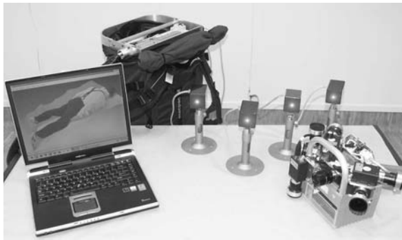
Figure 4: Scanner prototype: On the table from left to right are the base station, active targets which would be placed around the scene before the survey, and the scanner head. The scanner head is connected by umbilical cord to a processor-filled backpack.
