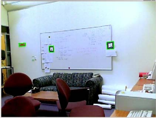
Figure 1: Two ARToolkit markers being used to calculate camera position. Markers are equal distances from ceiling and floor, and also the walls and each other.
