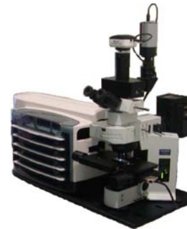
Figure 3: Microscope (right) with robotic slide loader (left).
