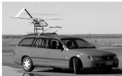
Figure 1: An Australian built Aerosonde UAV mounted for a car assisted launch. The sensor payload (currently under construction by Tenix Defence) is designed to fit in the front section of the fuselage.
