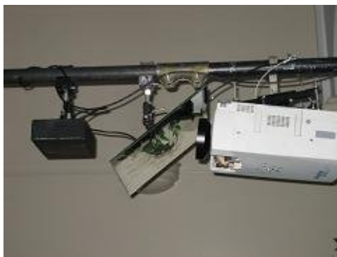
Figure 2. The projection reflects off a mirror onto the ground. Courtesy of LDPS NZ Ltd.
